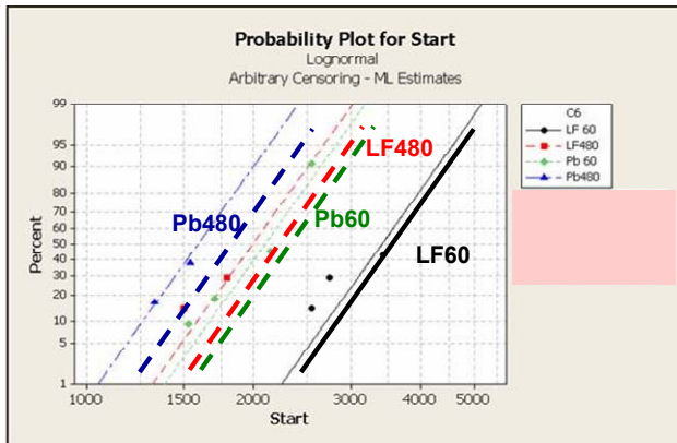
Figure 6: LF Temp cycle performance in long dwell time testing
